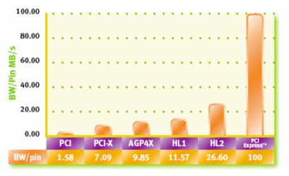
PCI @ 32b x 33MHz and 84 pins, PCI-X @ 64b x 133MHz and 150 pins, AGP4X @ 32b x 4x66MHz and 108 pins, Intel\* Hub Architecture 1 @ 8b x 4x66MHz and 23 pins; Intel Hub Architecture 2 @ 16b x 8x66MHz and 40 pins; PCI Express™ @ 8b/direction x 2.5Gb/s/direction and 40 pins.
